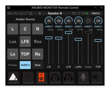
The AMBEO 2-Channel Spatial Audio live renderer unlocks investments into surround and immersive content for all viewers. Pictured is the prototype of the renderer interface for fine-tuning the spatially enhanced two-channel mix, controlled via the standard Anubis remote control software
